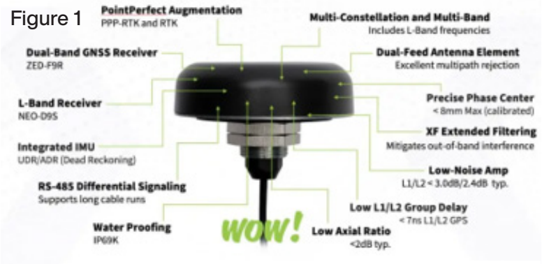
TW5390 Smart GNSS Antenna with IP-Network/L-Band Corrections and IMU
